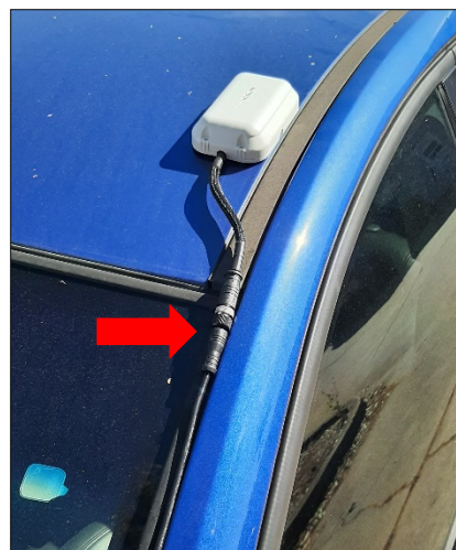
Satellite unit located on roof.
