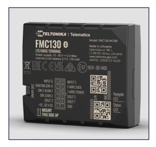
The FMC130 can be mounted under the plastic panel behind the front window, with the sticker/engraving direction to a window (sky). It is recommended to place FMC130 behind the dashboard as close to the window as possible.
